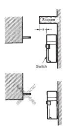
Refer to page 7 for the mounting dimensions of the Operation Key. Be sure that the Operation Key can be inserted properly with a tolerance of ±1 mm in the upward, downward, left, or right direction, otherwise the D4DS may be damaged.
