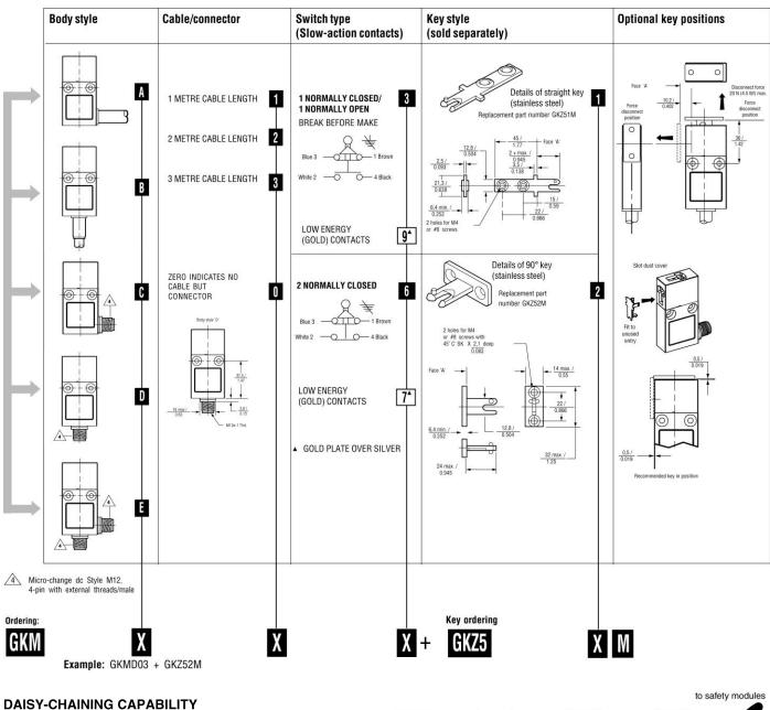
The GKME modules may be daisy-chained and terminated into either a GKMC or GKMD (as shown) for multi-door modular machinery.
