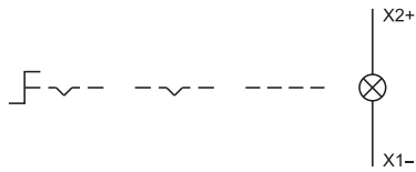
19 Selector switch actuator 3 positions, flush mounting page 11
