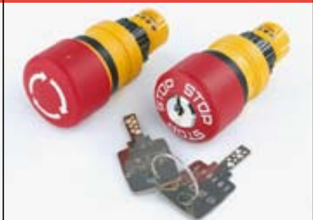
Emergency-stop, twist release and key release, 27 mm diameter for 16 mm mounting, foolproof to EN 60947-5-5 and DIN EN ISO 13850
