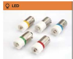
LED, BA9s (T-33/4 bayonet base), single chip, 28 Volt and 230 Volt. Also available in 6 Volt, 12 Volt, 24 Volt, 48 Volt and 230 Volt
