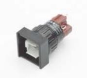
Illuminated pushbutton actuator, snap-action, raised, square, black plastic, 16mm mounting, solder terminals, gold over silver contacts
