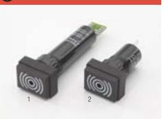
Buzzer, plastic bezel, raised, rectangular, 16mm mounting, continuous or intermittant tone, 88dB ± 8 at a distance of 0.1m
