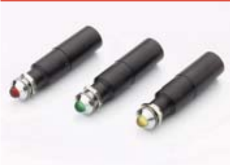
Indicator, external reflector, 5mm LED, 230VAC, 8mm mounting
