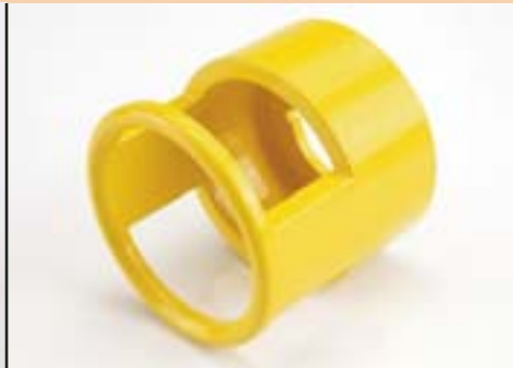
Emergency-stop protective shroud, yellow painted aluminium with 22.5mm mounting hole
