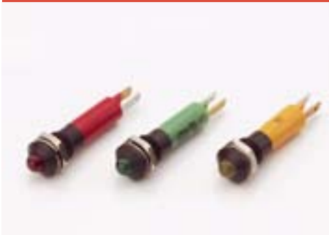
Indicator, external reflector, 5mm LED, 24VDC, 8mm mounting
