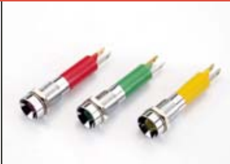
Indicator, internal reflector, 5mm LED, 24VDC, 8mm mounting
