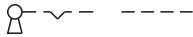
17 Keylock switch actuator 2 positions page 15 | Keylock switch actuator 2 positions, flush mounting page 21
