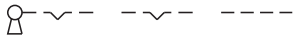
19 Keylock switch actuator 3 positions page 16 | Keylock switch actuator 3 positions, flush mounting page 22
