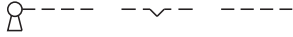
15 Keylock switch actuator 3 positions page 16 | Keylock switch actuator 3 positions, flush mounting page 22
