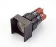
Illuminated pushbutton, snap-action, raised, square, black plastic, 16mm mounting, solder terminals, gold over silver contacts
