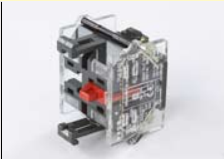
Switching element, screw terminal, snap-action with silver self-cleaning contacts
