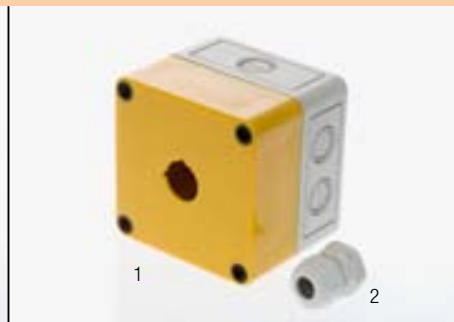
Emergency-stop switch enclosure 94 mm (w) x 94 mm (h) x 81 mm (d), anti twist hole. Cable gland M20, IP66
