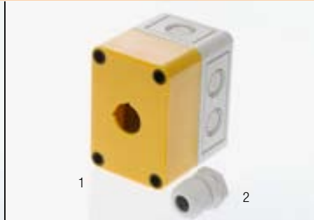
Emergency-stop switch enclosure, with 22.5 mm \varnothing mounting hole, 94 mm (w) x 65 mm (h) x 81 mm (d), anti twist hole. Cable gland M20, IP66
