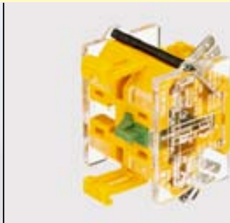
Switching element, plug-in terminal, 6.3 mm, snap-action with self-cleaning silver contacts
