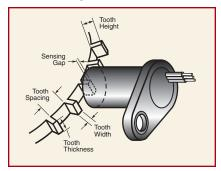
For best results, we recommend targets made from low carbon cold rolled steel. Other factors that influence sensor performance include geartooth height and width, space between teeth, shape of the teeth and thickness of the target. As a general guideline, consider a target with the following minimum parameters:
