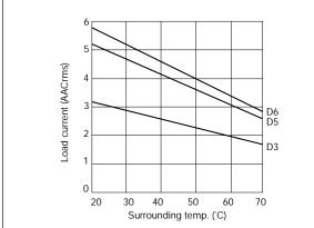
Derating curve is used for finding max. load current at an elevated ambient temperature. The 3 lines in the graph represent the 3 nominal current ratings of the RP1 series (RP1...D3/D5/D6).
