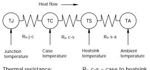
Thermal resistance:  $R_{th}j$ -c = junction to case  $R_{th}$  c-s = case to heatsink  $R_{th}$  s-a = heatsink to ambient
