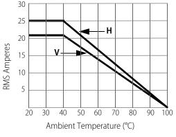
V. Heatsink mounted to a **vertical** surface H: Heatsink mounted to a **horizontal** surface.
