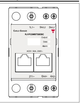
All dimensions in mm Note: Terminals 5N/L2 and 3N/L2 are available only on RJ1P23MBT50ECV
