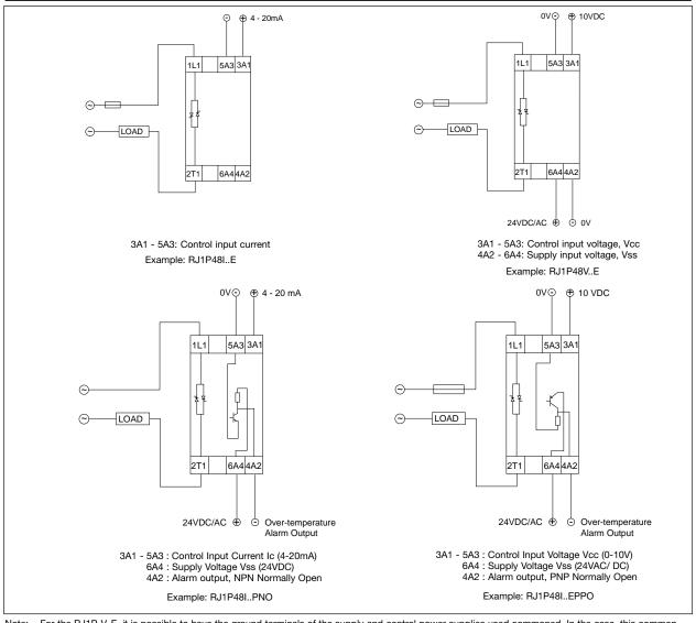
Note: For the RJ1P.V.E, it is possible to have the ground terminals of the supply and control power supplies used commoned. In the case, this common ground is connected either to terminal A2 or terminal A3. This is only applicable when a 24 VDC supply voltage is used. There should be no external direct link from Terminal A2 to Terminal A3.
