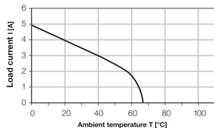
The solid-state relay **MICROOPTO ACTOR** has been especially designed as a switching amplifier for actuators up to 24VDC and 2A with inductive loads such as solenoid valves and contactors. 3-wire actuators can be connected directly to the module.
