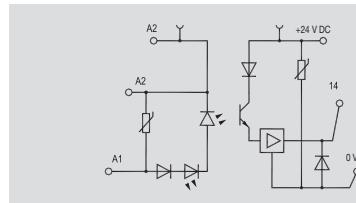
A special integrated circuit in the opto module **MICROOPTO 100 kHz** ensures that rapidly transmitted signals are isolated from one another and that they can be transferred practically without delay. This allows switching frequencies up to 100 kHz to be achieved.
