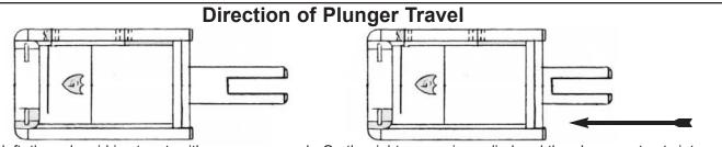
On the left, the solenoid is at rest, with power removed. On the right, power is applied and the plunger retracts into the body of the solenoid in the direction of the arrow. Optional spring kits return plunger to the "rest" position.
