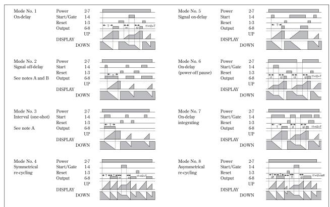
Notes: A In modes 2 and 3, after the time is up and the output turns off, a reset signal is not required before another start signal is given. The start signal itself will also effect a reset first.
