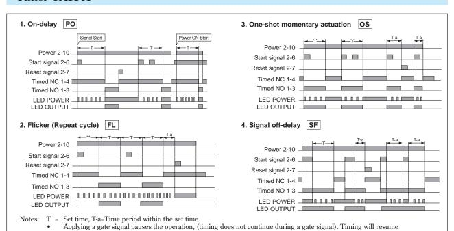
at the point where it left, as soon as the gate signal is removed. Each signal can be input by short circuiting the relevant terminals. Power LED lights up when power is ON, but flickers during timing.
