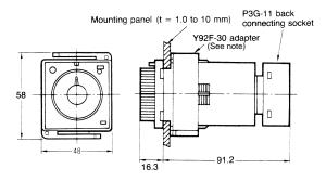
**Note:** The adapter can be mounted to the timer form any side of the timer housing since the adapter security notches are provided on all four sides of the housing.
