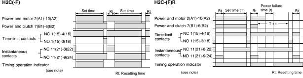
Note: For the types rated at 24 and 48 VAC, the timing operation indicator is not equipped.
