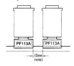
**Note:** For a load current of 3 A max., a spacer and an end plate are not required. For a load current of 6 A, one spacer or an end plate is required.
