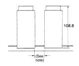
Note: For a load current of 1 A max., a spacer and an end plate are not required. For a load current of 3 A max., one spacer or an end plate is required. For a load current of 6 A max. two spacers or two end plates are required.
