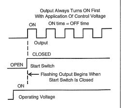
The timing diagram shown below is for an application that requires the load circuit to be ON for 60 milliseconds and OFF for 60 milliseconds. (Remember - the ON and OFF times will essentially be equal due to the 50% duty cycle specification inherent in the model 423)
