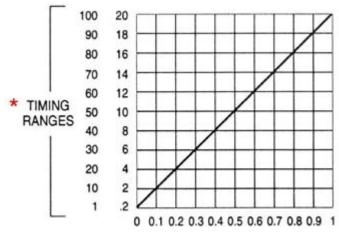
TIMING RESISTOR IN MEGOHMS
