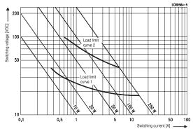
Load limit curve 1  $\triangleq$  arc extinguishes, during transit time (changeover contact)
