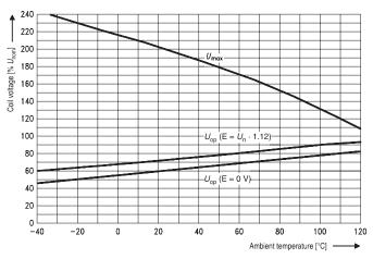
Does not take into account the temperature rise due to the contact current  $\mathsf{E} = \mathsf{pre}\text{-energization}$
