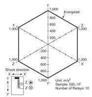
Conditions: Shock is applied in  $\pm X$ ,  $\pm Y$ , and  $\pm Z$  directions three times each with and without energizing the Relays to check the number of contact
