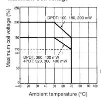
The maximum coil voltage refers to the maximum value in a varying range of operating power voltage, not a continuous voltage.
