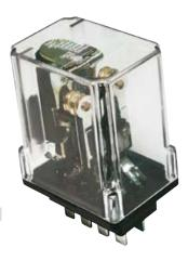
The 21 series coil is rectified which provides chatter free operation in brownout conditions down to 85VAC and will not overheat up to 130VAC. Rectified coils also provide less power consumption and less heating.
