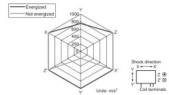
Measurement conditions: Impose a shock in the  $\pm X$ ,  $\pm Y$ , and  $\pm Z$  directions three times each with the Relay energized to check the shock values that cause the Relay to malfunction.
