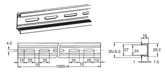
A total of twelve  $25 \times 4.5$  elliptic holes is provided with six holes cut from each track end at a pitch of 10 mm.
