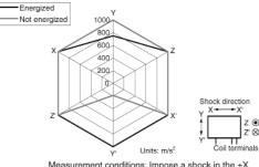
Measurement conditions: Impose a shock in the  $\pm X$ ,  $\pm Y$ , and  $\pm Z$  directions three times each with the Relay energized to check the shock values that cause the Relay to malfunction.
