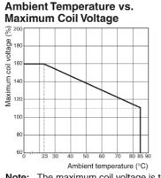
Note: The maximum coil voltage is the maximum voltage that can be applied to the relay coil
