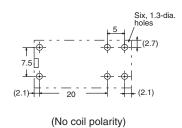
**Double-winding Latching Relays with PCB Terminals**
