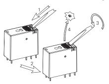
A standard XT series relay with a test lever is delivered with the locking function of the test lever disabled. In this state, a small plastic nib is designed to interfere with the lever moving to the locking position in normal operation; however, if the test lever is moved too forcefully, it may bypass the normal test position and go to the locked position.
