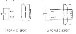
NOTE: Observe coil polarity on models with the optional protection diode. A1 is positive and A2 is negative.
