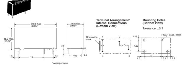
ALL DIMENSIONS SHOWN ARE IN MILLIMETERS. To convert millimeters into inches, multiply by 0.03937. To convert grams into ounces, multiply by 0.03527.
