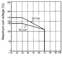
The maximum coil voltage refers to the maximum value in a varying range of operating power voltage, not a continuous voltage. Note:
