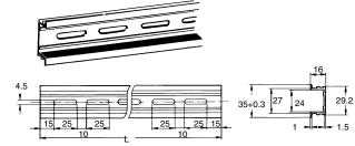
It is recommended to use a panel 1.6 to 2.0 mm thick.
