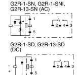
(After confirming coil polarity, wire correctly.) (Except G2R-1-S, G2R-13-S)
