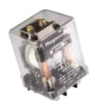
The 785 Magnetic Latching relay, with an Industry Standard square base, operates by using a pulsed input. A permanent magnet maintains the last position until a redirected second pulse moves the contacts back to the original state.
