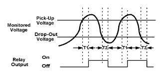
period longer than the adjustable pick-up time delay (T1) of 0.1-10 seconds. The relay de-energizes when the monitored voltage is below the drop-out setting for a period longer than the drop-out time delay (T2), which is adjustable from 0.1-10 seconds. The pick-up time (T1) and drop-out time (T2) are independently adjustable.
