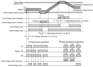
Note: 1. The K8AB-PM output relay is normally operative.
