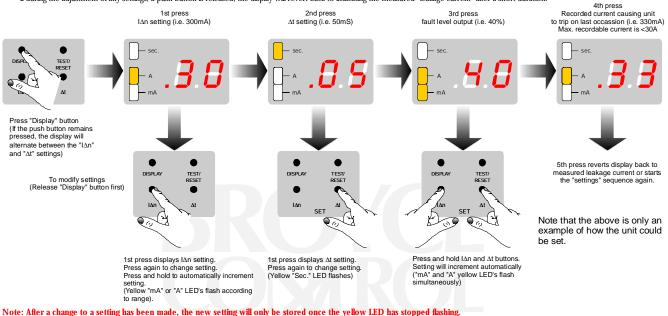
Fault simulation (Test mode)
