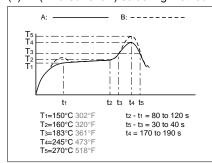
Temperature rise of relay itself may vary according to the mounting level or the heating method of reflow equipment. Therefore, please set the temperature of soldering portion of relay terminal and the top surface of the relay case not to exceed
