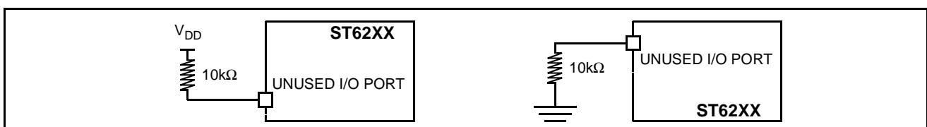
Figure 62. Two typical Applications with unused I/O Pin
