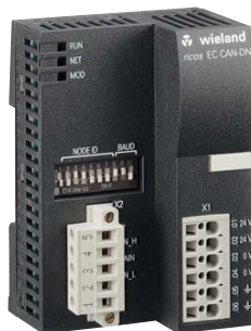
Modular economy buscoupler DeviceNet CE; Approvals: \text{UL} in preparation
