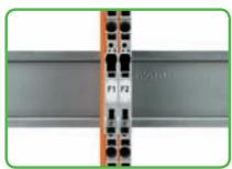
Fuse terminal blocks with a width of 6.2 mm/0.244 in can be assembled adjacent to each other. At the end of an assembly, if there is **no** adjacent fuse or disconnect terminal block, an end plate for fuse terminal blocks must be used.
