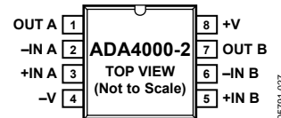
Figure 3. 8-Lead SOIC (R-8)
