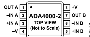
Figure 4. 8-Lead MSOP (RM-8)
