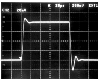
TPC 21. Small Signal Pulse Response, G = +5 , R_L = 20 k\Omega , C_L = 50 pF
