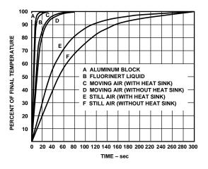
Figure 8. Thermal Response Curves
