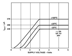
Figure 1. V-I Characteristics
