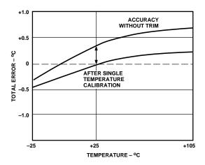
Figure 5. Effect of Scale Factor Trim on Accuracy
