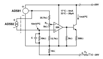
Figure 12. Temperature to 4–20 mA Current Transmitter
