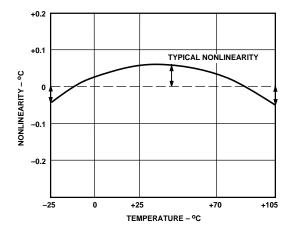
Figure 3. Nonlinearity Error (AD592CN)
