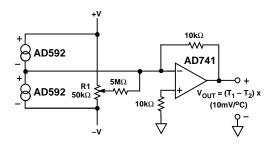
Figure 10. Differential Measurements
