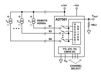
Figure 15. Remote Temperature Multiplexing
