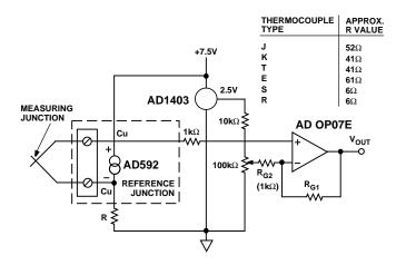
Figure 11. Thermocouple Cold Junction Compensation
