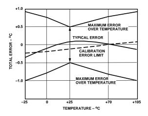
Figure 2. Error Specifications (AD592CN)
