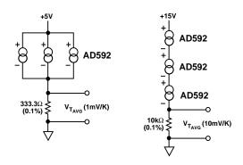
*Figure 9. Average and Minimum Temperature Connections*
