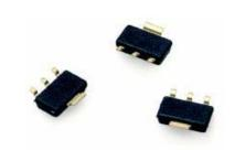
SS552MT is a digital position sensor in an SOT-89 style surface-mount package with omnipolar magnetic action. The sensor has magnetoresistive material integrated on silicon and encapsulated in a plastic package. The integrated circuit provides a digital output in response to very low magnetic fields. Though this signal is identical to our digital Hall effect sensors, it can be achieved by magneto-resistive sensors at much greater sensor-to-magnet distances.
