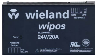
24 V / 20 A Three-phase primary switch-mode regulator CE; Approvals: and CSA pending 240 x 130 x 86
