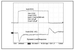
**FIGURE 2-29:** Dynamic Load Response (10 mA to 500 mA).
