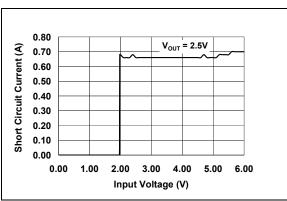
FIGURE 2-21: Short Circuit Current vs. Input Voltage.
