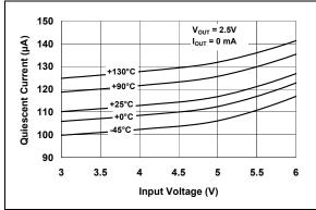
FIGURE 2-11: Quiescent Current vs. Input Voltage.
