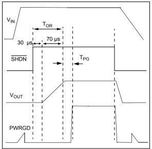
**FIGURE 4-3:** Power Good Timing from Shutdown.
