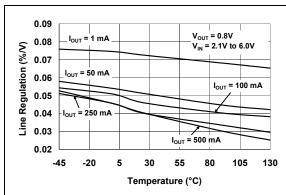
FIGURE 2-15: Line Regulation vs. Temperature.
