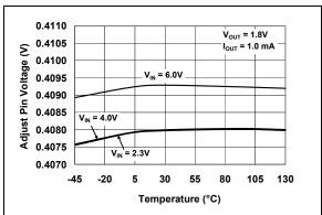
FIGURE 2-6: Adjust Pin Voltage vs. Temperature (Adjustable Version).
