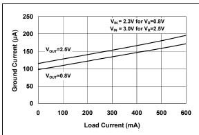
FIGURE 2-12: Ground Current vs. Load Current.
