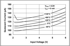
FIGURE 2-10: Quiescent Current vs. Input Voltage.
