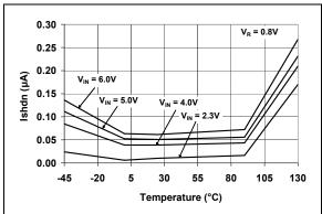
FIGURE 2-14: I<sub>SHDN</sub> vs. Temperature.
