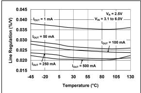
**FIGURE 2-16:** Line Regulation vs. Temperature.
