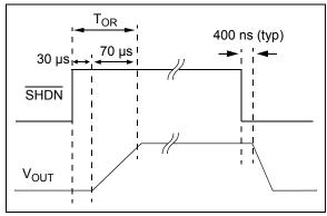
FIGURE 4-4: Shutdown Input Timing Diagram.
