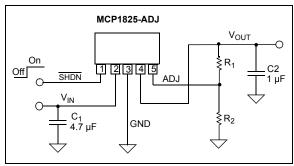
**FIGURE 4-1:** Typical adjustable output voltage application circuit.
