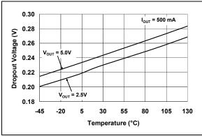
FIGURE 2-20: Dropout Voltage vs. Temperature.
