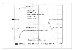
**FIGURE 2-30:** Dynamic Load Response (100 mA to 500 mA).
