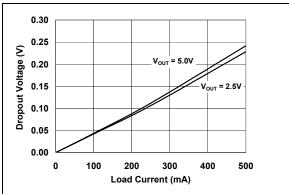
FIGURE 2-19: Dropout Voltage vs. Load Current.
