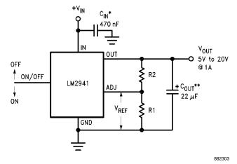
$$V_{OUT} = \text{Reference voltage} \times \frac{\text{R1} + \text{R2}}{\text{R1}} \text{ where } V_{REF} = 1.275 \text{ typical}$$
