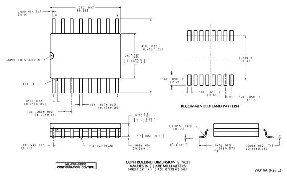
Order Number LM2941WG/883 LM2941WG-QMLV, 5962-9166701QYA NS Package Number WG16A
