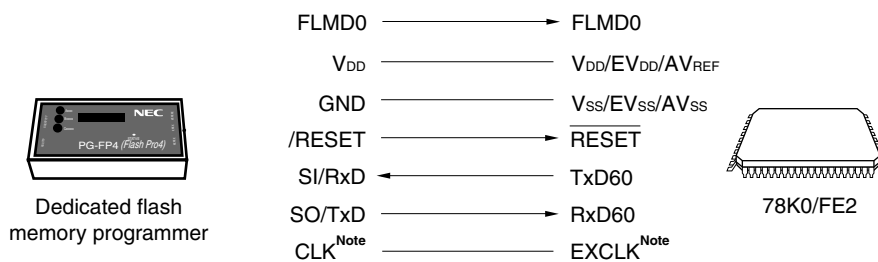
Figure 24-7. Communication with Dedicated Flash Memory Programmer (UART60)
