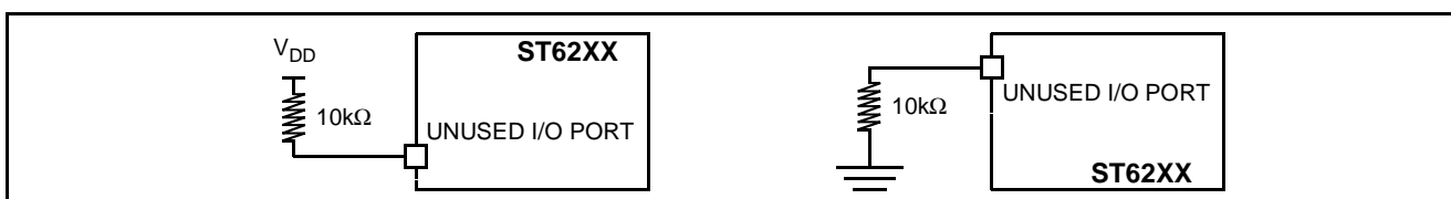
Figure 62. Two typical Applications with unused I/O Pin
